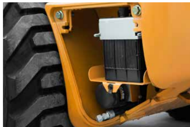
Smart battery and drain hoses access Battery and environmental drain hoses are easily accessible from the side of the machine, by removing a tap located behind the rear wheel, allowing quick service and fast maintenance activities.
