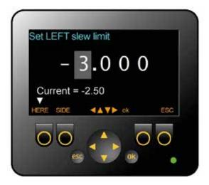
A slew limit can be either manually keyed in or set automatically by positioning the machine equipment and pressing HERE.
