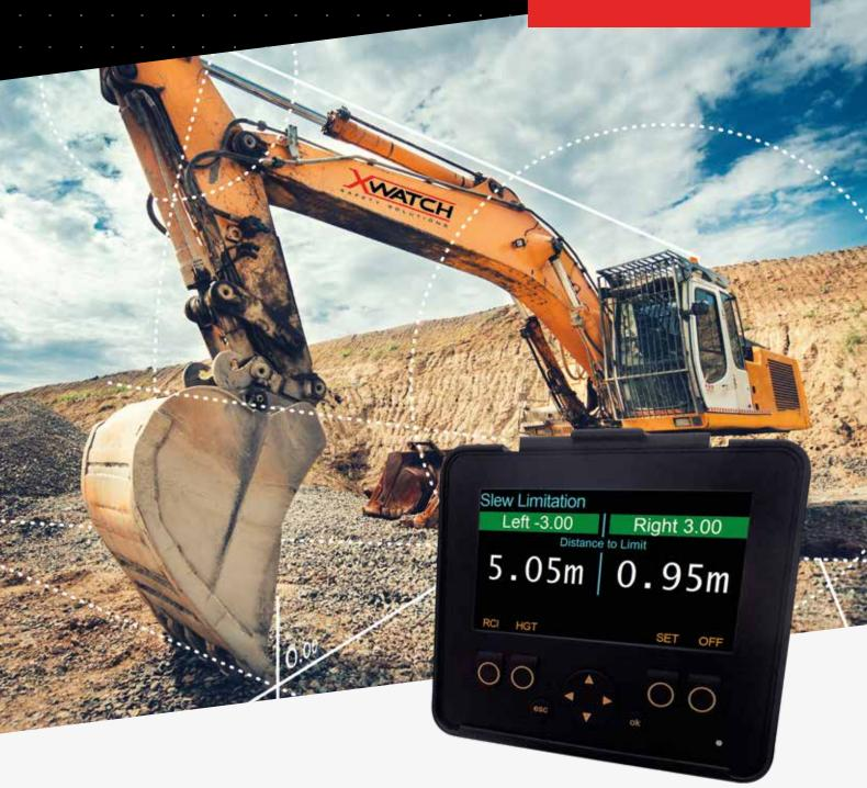
The XW3 can be configured to work on a variety of articulated hydraulic plant. Slew limitation is controlled using proportional soft-stop hydraulic valves providing accurate and repeatable performance without detriment to the machine.
