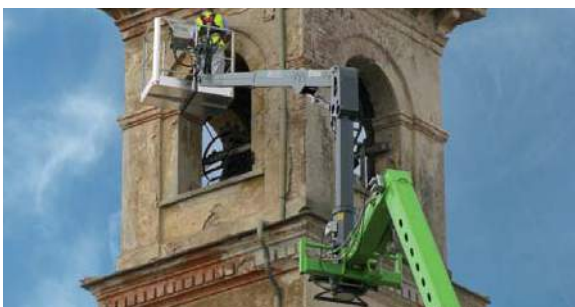
The swing of the Space System platform handling boom allows access to points that would otherwise be difficult to reach
