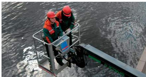
Regardless of the type of platform being used, the operator controls all movements from on board the platform
