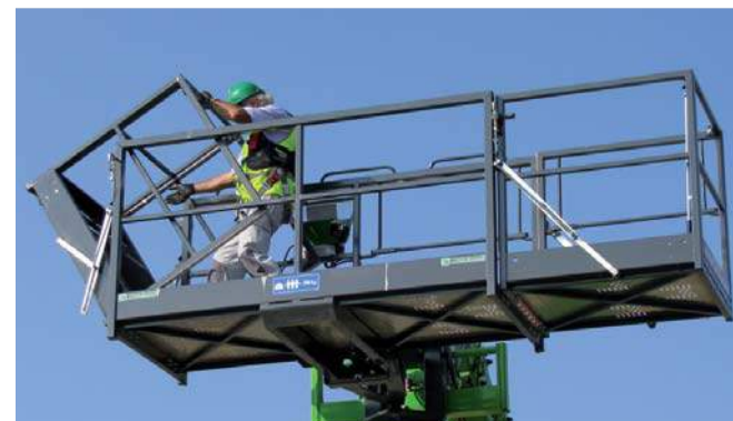
In some Merlo overhead platforms, the useful width is variable, thanks to the practical and patented extension system, which can be operated even at height
