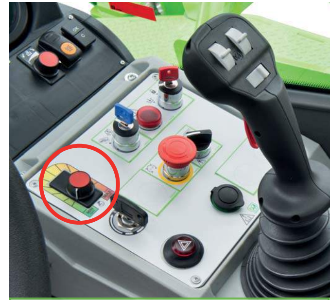
Potentiometer to manually set diesel engine rpm
