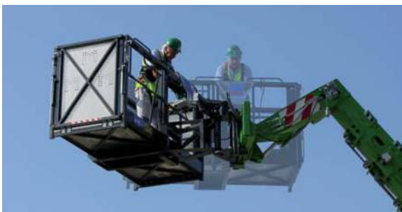
The hydraulic rotation around the vertical axis of many Merlo overhead platforms allows work with the machine tilted
