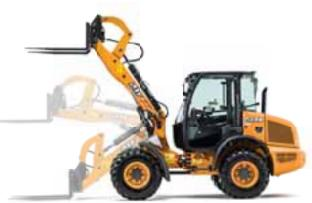
XT is the best linkage for pallet handling. Visibility on the pallet is the best with one lifting cylinder only and payload is optimum
